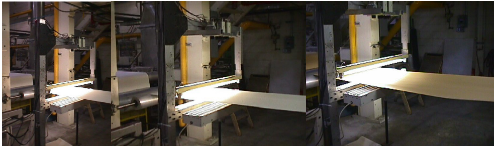
Figure 34 - Showing the web sagging problem during the Newsprint A trial run that contributed to web breaks.
