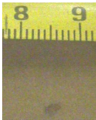
Figure 26 - Picture of spot defect detected during linerboard import test run
