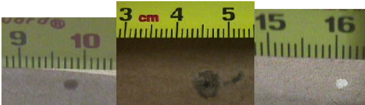
Figure 28 – Pictures of defects detected at production speed during the 33-lb Linerboard Export Test. Defects include a light spot, oil and type of scale
