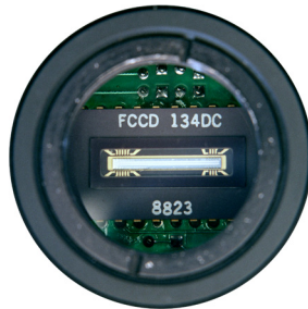
Figure 1 – 2048 Pixel Line Scan CCD Chip
