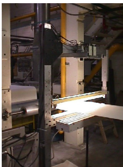
Figure 22 - View of newsprint roll A sagging prior to inspection due to excessive web flutter
