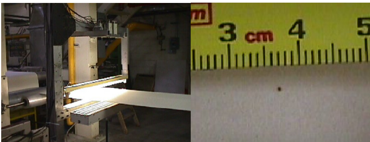
Figure 39 - Camera frame during testing of Newsprint Roll B and a spot defect detected during the run.
