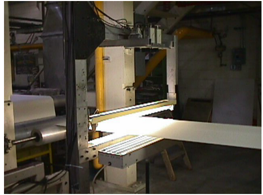
Figure 17 - Placement of lighting across pilot coater and paper web
