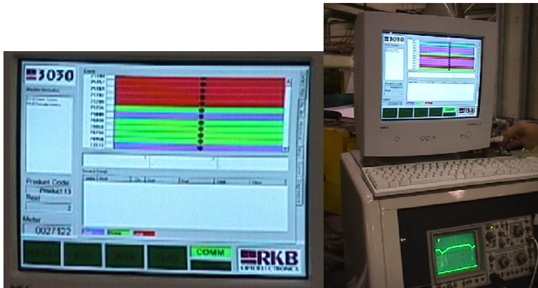
Figure 33 - View of cabinet and CRT screen during trial with calibrated defects. Each Red strip indicates a large size defect, Green medium and Blue small.
