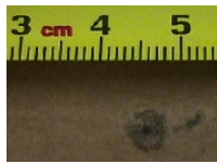
Scale 33-lb linerboard @ 2500 feet/min (762 m/min)
