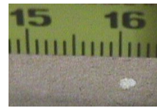
Light Spot 33-lb linerboard @ 2500 feet/min (762 m/min)
