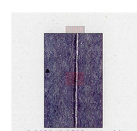
0.002" (0.0508mm) wide 220# CN COVER @ 1200 fpm (365 m/min) One Coating Scratch Detected by the OPTOMIZER
