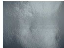
Coating Streak (silicone coating)
