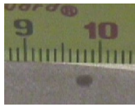
Black Spot 33-lb linerboard @ 2500 feet/min (762 m/min)
