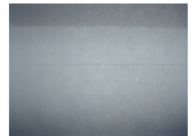
Coating Streak (silicone coating)
