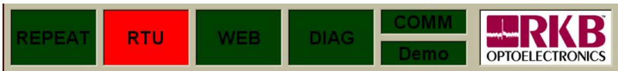
System Diagnostic Alarm Indicators (show reel turn up alarm indication)
