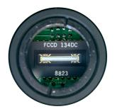
Figure 1 – 2048 Pixel Line Scan CCD Chip
