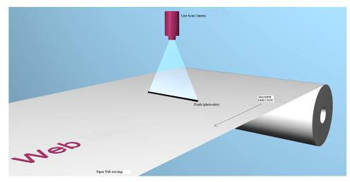
Figure 5 – Machine Direction pixel resolution on a moving web or "Dynamic Resolution"
