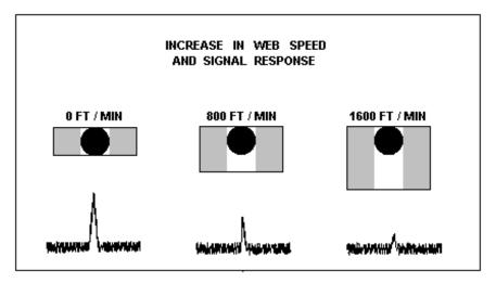
Figure 8 – Effects of web speed on the defect signal to noise ratio
