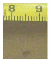
Figure 26 - Picture of spot defect detected during linerboard import test run
