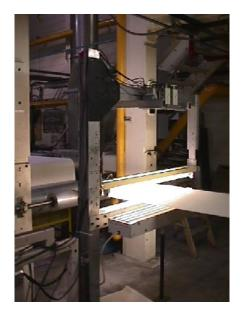
Figure 22 - View of newsprint roll A sagging prior to inspection due to excessive web flutter
