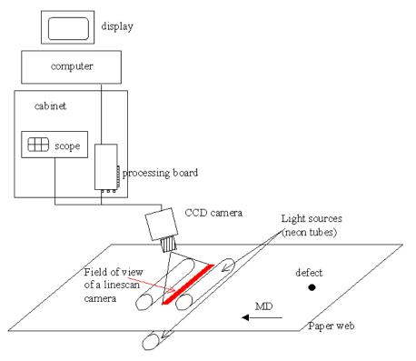
Figure 11 - Diagram of RKB 3030 for discrete defect detection
